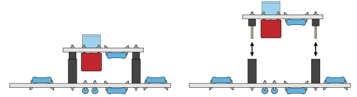
It's done in this order so that that the pins are perfectly coupled with the headers. If they were soldered separately from each other, the slight misalignments between the pins and headers would create stress that could potentially cause cracked solder joints over time.
