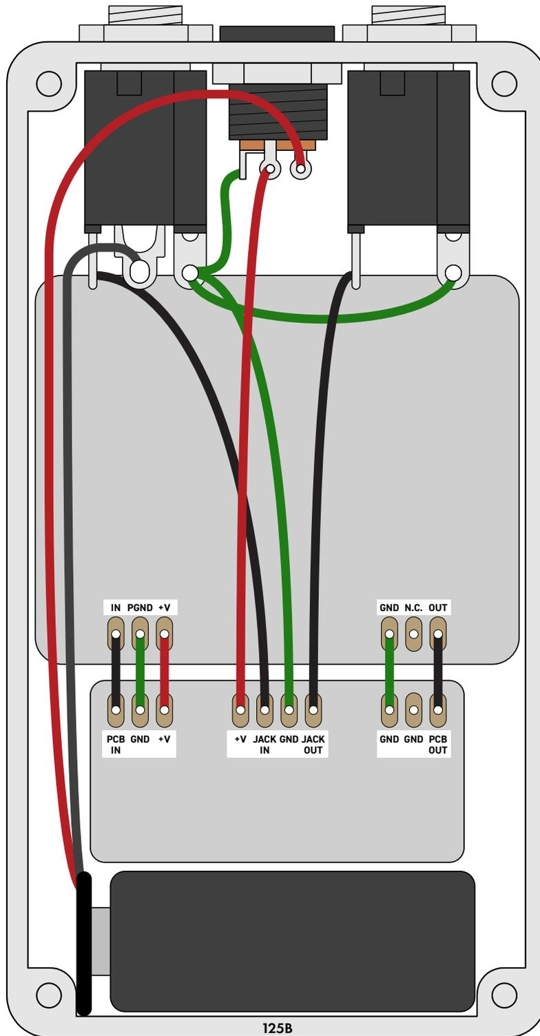
*Shown with optional 9V battery. If battery is omitted, both jacks can be mono rather than one being stereo.
