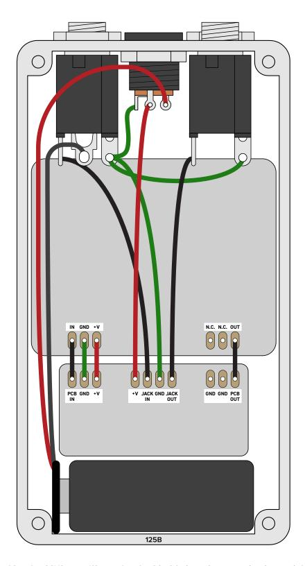
Shown with optional 9V battery. If battery is omitted, both jacks can be mono rather than one being stereo. Leave the far-right lug of the DC jack unconnected.
