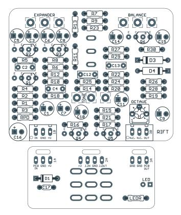
Actual size is 2.3" x 1.86" (main board) and 2.3" x 0.86" (bypass board).
