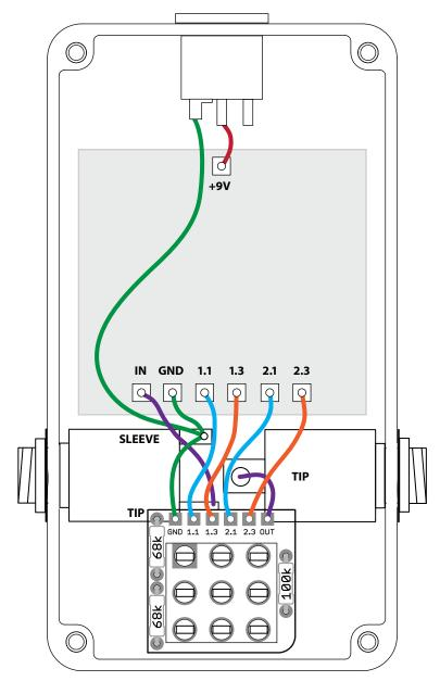
Wiring is dead simple: the pads match up to the Aion Refractor PCB project, so you can run the wires straight across (as shown in the diagram to the left) and be done with it. But here's a description of each of them.
