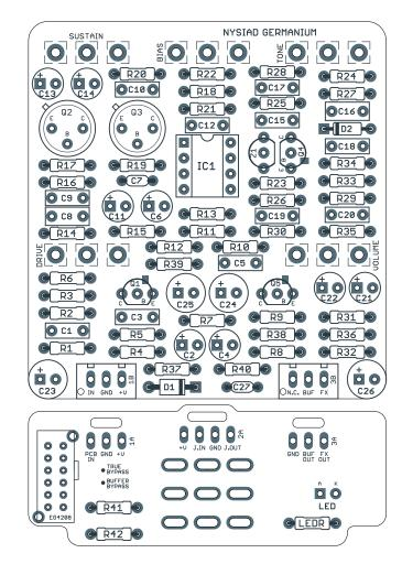
Actual size is 2.3" x 2.43" (main board) and 2.3" x 0.87" (bypass board).
