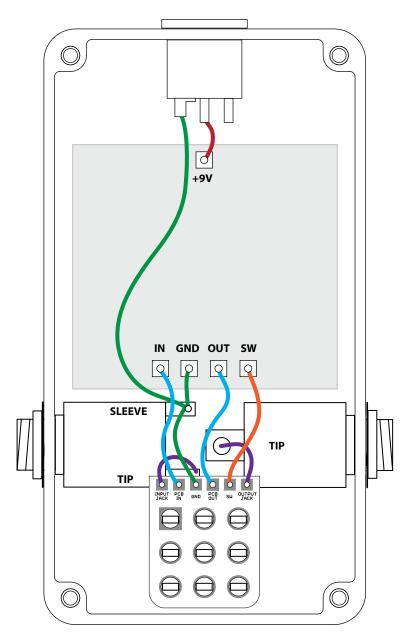
Wiring is dead simple: the pads match up to every Aion PCB project, so you can run the wires straight across (as shown in the diagram to the left) and be done with it. But here's a description of each of them.
