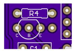
Assuming E-B-C pinout, you just shift it to the left by 1 pin from where the JFET would normally go.
