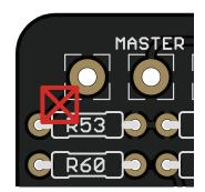
Both of these loops have an additional 51R resistor that is shown in the wiring diagram between the Send and Return jacks. The way it's wired, this resistor is in series with the only Send jack of each loop, and is out of the circuit entirely when nothing is plugged into the Return jack.
