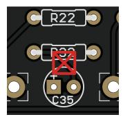
R32 (jumper), C35 (10uF) and R33 (100k) should still be installed as normal. The wires need to share the pads with the components. The easiest method is to elevate the resistor above the PCB slightly before soldering and then solder the wire underneath the lifted leg.
