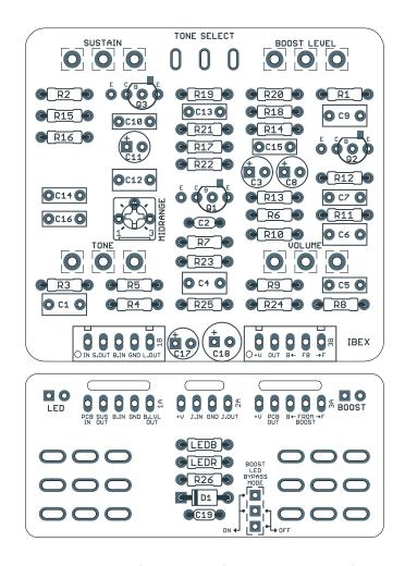
Actual size is  $2.3" \times 2.14"$  (main board) and  $2.3" \times 1.05"$  (bypass board).
