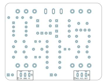
Install the two 3-pin headers (wire connectors) as shown above. These have a polarity pin, so as long as they are pressed all the way down, there's only one possible way to install them. They do fit pretty tightly in the holes, though, so press firmly.
