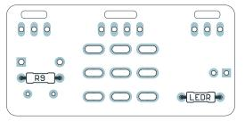
Using the parts list above, populate the resistors by pushing them through the holes and bending the leads outward at an angle to hold them in place. Resistors are not polarized, so they will work in any direction. Turn the board upside-down to keep the components held in place while you solder.
