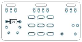
Next, you'll populate the diodes. Diodes are polarized, so make sure to identify the polarity band (which indicates the "cathode", or negative side) and match the band to the footprint on the PCB.
