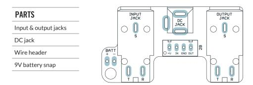
Almost done! Get the two input/output jacks, the DC jack and the wire header and snap them in place. The PCB is designed for them to fit securely, so you can do them all at once before flipping and soldering.
