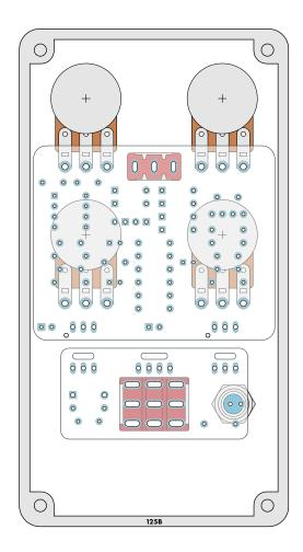
After all the components are affixed to the enclosure as shown on the previous page, place the main PCB on top of the potentiometers and toggle switches as in the diagram to the left.
