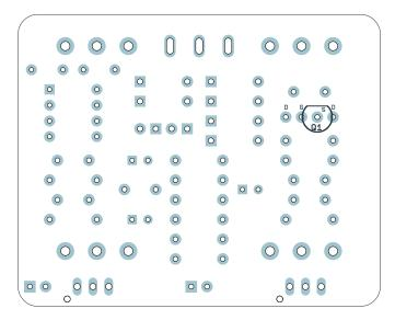
Now we'll do the JFET transistor. If the legs are not already bent into 0.1" spacing, use your needle-nose pliers to bend the outer two legs as shown.
