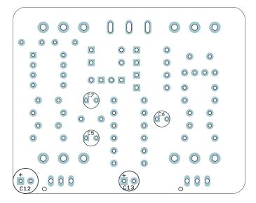
Populate the electrolytic capacitors. These are the tallest components so we save them for last. They are polarized (i.e. they will only work in one direction), so note the vertical mark on the capacitor that indicates the negative side. The longer leg is positive and fits in the square pad.
