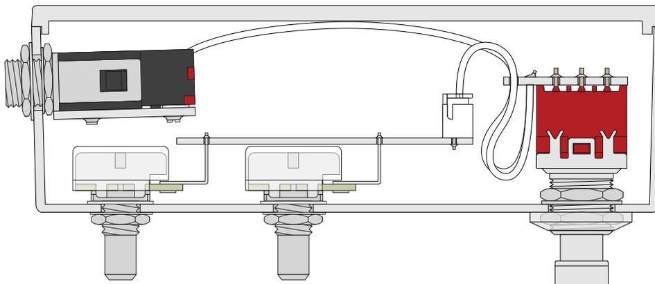
At this point, you have completed the full circuit as far as the electrons are concerned. Plug in a 9-volt supply and test it out with a guitar and an amplifier. It's recommended to use the starting knob positions on the next page if you're not familiar with the Fuzz Factory circuit.
