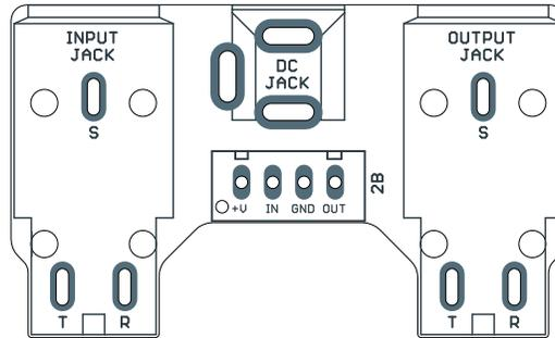
Almost done! Get the two input/output jacks, the DC jack and the wire header and snap them in place. The PCB is designed for them to fit securely, so you can do them all at once before flipping and soldering.
