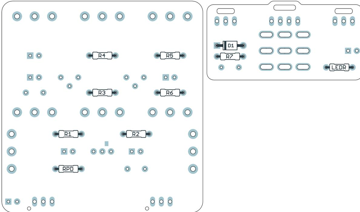
Using the parts list above, populate the resistors and diode by pushing them through the holes and bending the leads outward at an angle to hold them in place. Resistors are not polarized, so they will work in any direction, but note that the diode is polarized and must be installed with the silver band lining up with the band on the PCB silkscreen.
