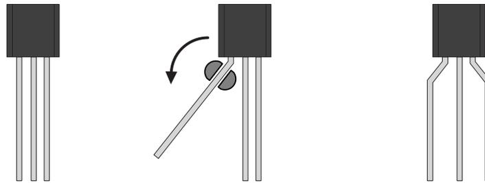
Bend the outer leads of the transistor to hold it in place on the board. Then, solder it and clip the leads.
