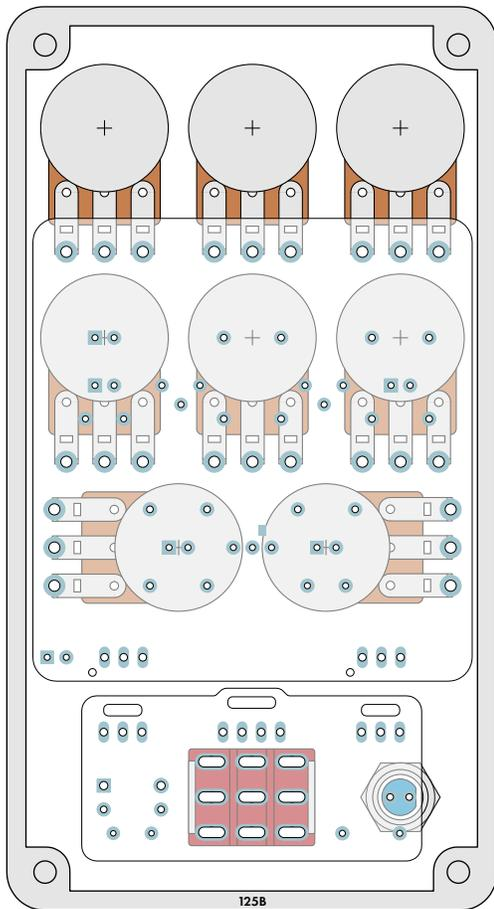
After all the components are affixed to the enclosure as shown on the previous page, place the main PCB on top of the potentiometers as in the diagram to the left.
