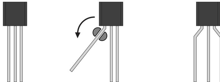
Bend the outer leads of the transistor to hold it in place on the board. Then, solder it and clip the leads.
