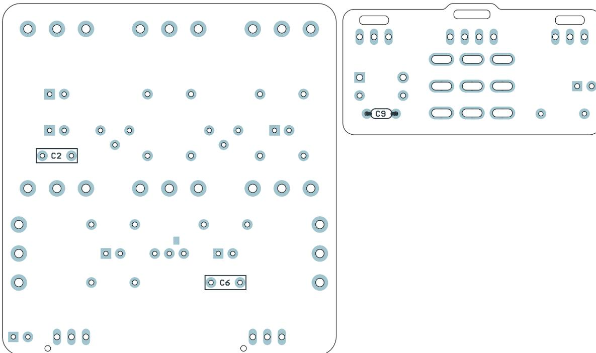
After the silicon transistor come the box film and MLCC capacitors. As with previous components, bend the leads at an angle to hold them in place.
