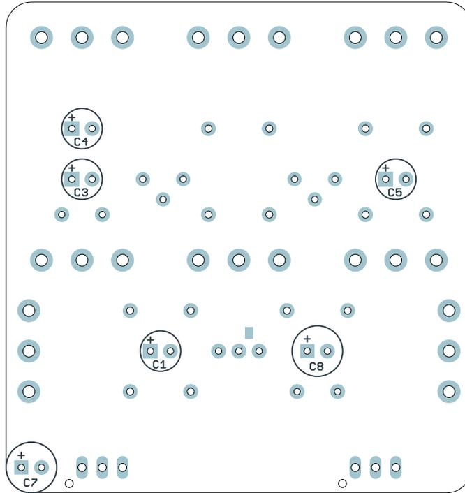
Populate the electrolytic capacitors. They are polarized (i.e. they will only work in one direction), so note the vertical mark that indicates the negative side. The longer leg is positive and fits in the square pad.
