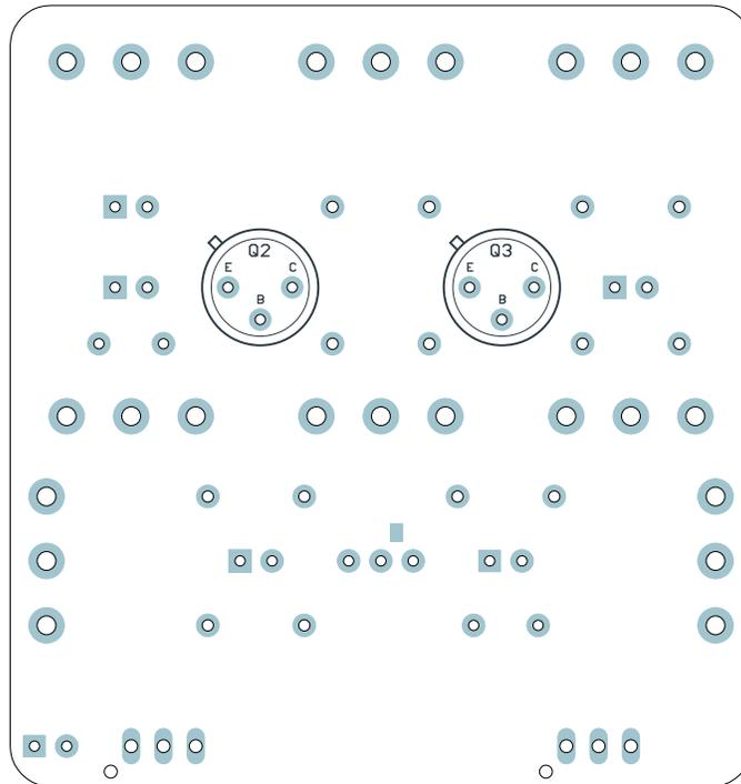
Now that we've covered the basics of germanium transistors, it's time to install them. Remove Q2 (the front transistor with a lower gain value) from the bag. As mentioned on the previous page, it's important to leave Q3 in its bag until Q2 has been soldered so they don't get mixed up.
