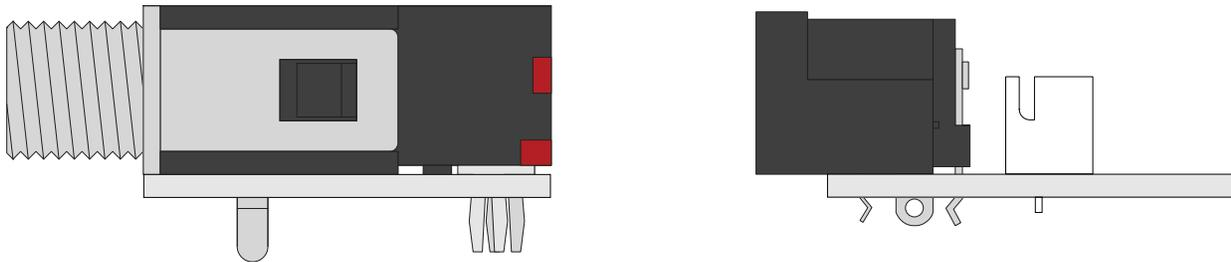
After you've soldered everything, make sure to **snip the leads on the I/O jacks as close as possible to the PCB**. There's not a lot of clearance between the bottom of this board and the top of the main PCB once everything is in place, and you don't want the pins to short against anything on accident.
