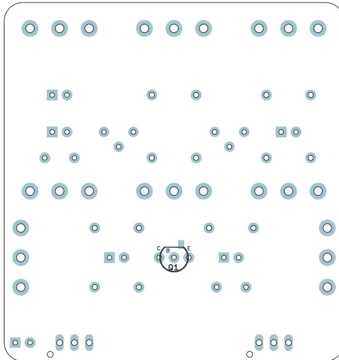
Now we'll do the silicon transistor. If the legs are not already bent into 0.1" spacing, use your needle-nose pliers to bend the outer two legs as shown.
