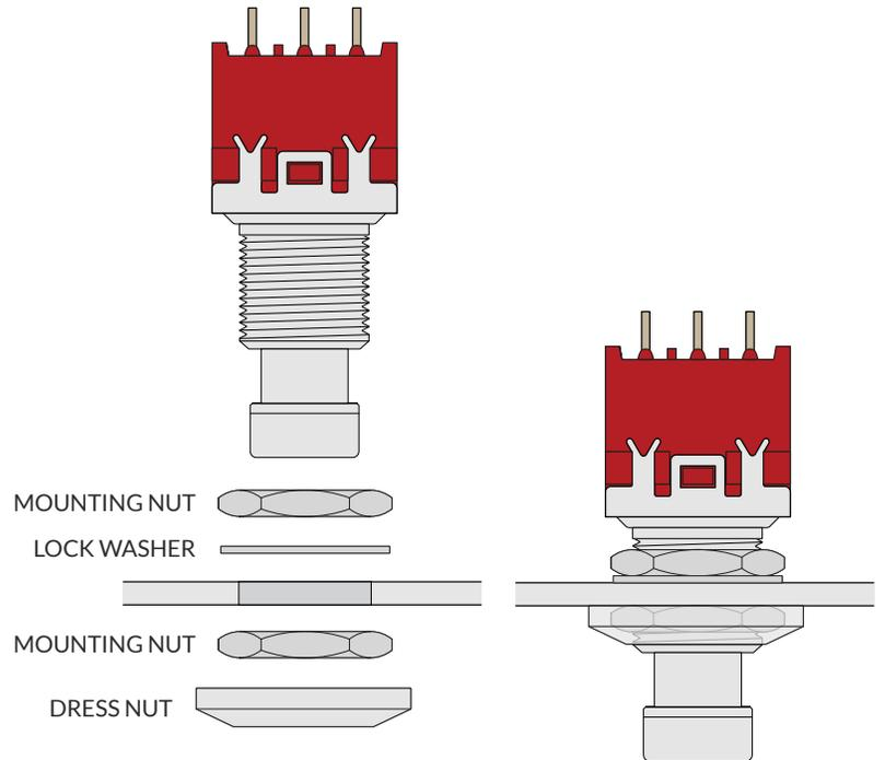
The dress nut fits over the top of the mounting nut and is for aesthetic purposes only. Wrap a rubber band around it to use as a grip when tightening. Avoid using metal tools on it or you run the risk of scratching or denting it.
