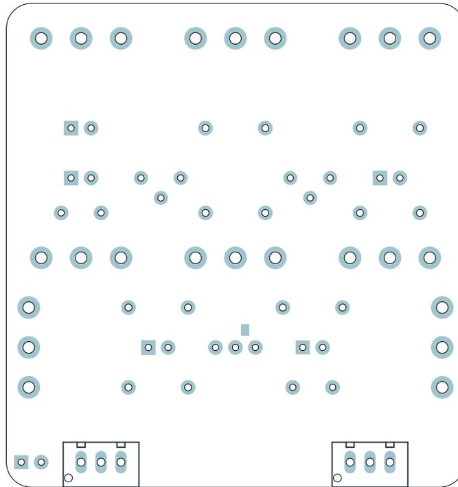
Install the two 3-pin headers (wire connectors) as shown above. These have a polarity pin, so as long as they are pressed all the way down, there's only one possible way to install them. They do fit pretty tightly in the holes, though, so press firmly.
