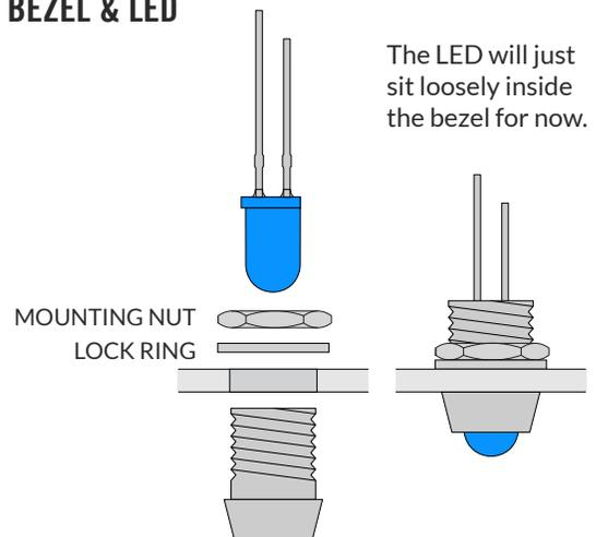
You'll need to hold the bezel in place when tightening the nut. The top of the bezel is fairly sharp, so try using a rubber band for grip instead of pressing your finger against the bottom.
