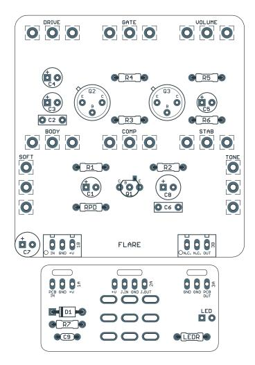
Actual size is  $2.3" \times 2.42"$  (main board) and  $1.78" \times 0.86"$  (bypass board).
