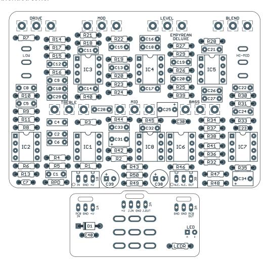
Actual size is 3.44" x 2.42" (main board) and 1.77" x 0.87" (bypass board).
