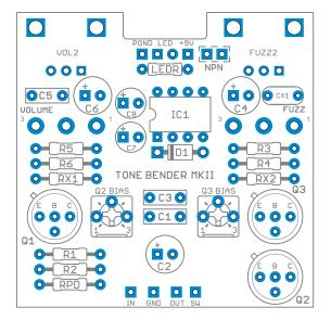
The Deimos Fuzz is a clone of the Tone Bender Mark 2 (twoknob). While the first version of the Tonebender was essentially a slightly tweaked Fuzz Face, the Mark 2 version added a singletransistor boost in front of it. But even though the topology is similar to a Fuzz Face, the biasing scheme is very different, and its optimum transistors are not the same as a Fuzz Face set.
