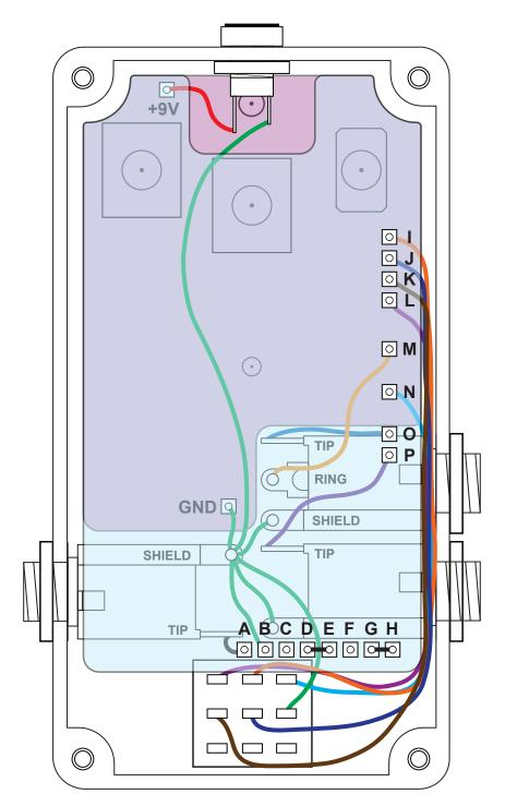
In this wiring diagram, pads C and F are left unconnected. Pads D & E and G & H are jumpered.
