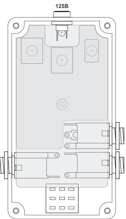
The **in/out jacks** are Switchcraft 111X for "In" and "Out A" and 112BX for "Out B". Clones of these can be found pretty easily and will work fine—but they must be the black box-style enclosed jacks, not the open-frame type (Switchcraft 11 / 12B) or Neutrik NMJ series.
