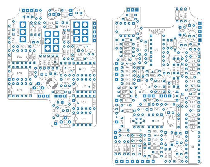
These are shown 50% bigger than life size. The PCB on the left (the clock + LFO board) measures 2.15" x 2.9". The PCB on the right (the signal board) measures 2.15" x 3.79". They are shown here with component sides facing up, but component sides will face down when installed in the enclosure.
