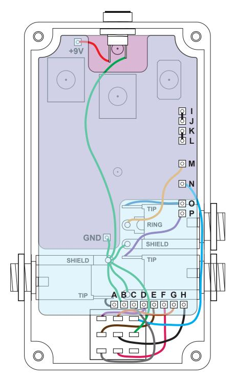
In this wiring diagram, pads I & J and K & L are jumpered.
