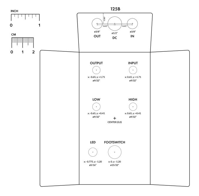
Enclosure is shown without jacks. See next page for jack layout and wiring.
