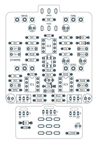
Actual size is 2.3" x 2.61" (main board) and 1.78" x 0.90" (bypass board).
